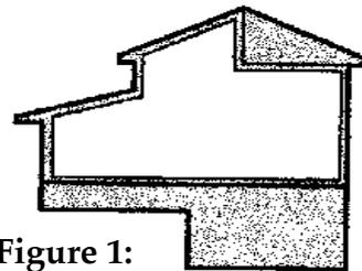
**Figure 1:** The ceiling, walls and floors between heated and unheated spaces form the air and insulation barriers of your home
